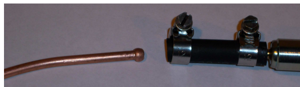
Flared end of copper pipe
